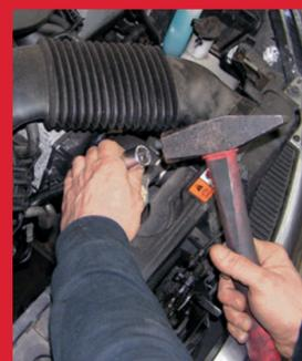
**Cockpit lights are on, starter motor starts the engine only tiredly.**
