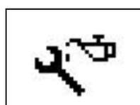
Diagnostic / Vehicle selection Icon – Select this to go into the Diagnostic menu for service related items or to clear fault codes via EOBD
