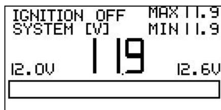
The status of battery voltage with the ignition off and engine off is displayed.
