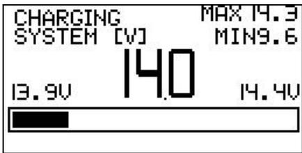
The status of battery when charging will be displayed once the alternator has stabilised.
