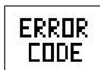
Error Code Icon – Select this to enter the EOBD (European On Board Diagnostics) software. This is included as standard on all European vehicles (from 2000 for petrol, from 2004 for diesel) and provides basic information and error codes relating to engine emissions.
